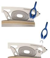
You can now change the blade-runner and shock-absorbers. Position the new shock-absorbers or blade-runner in the frame. Refer to the example picture for correct placement.
